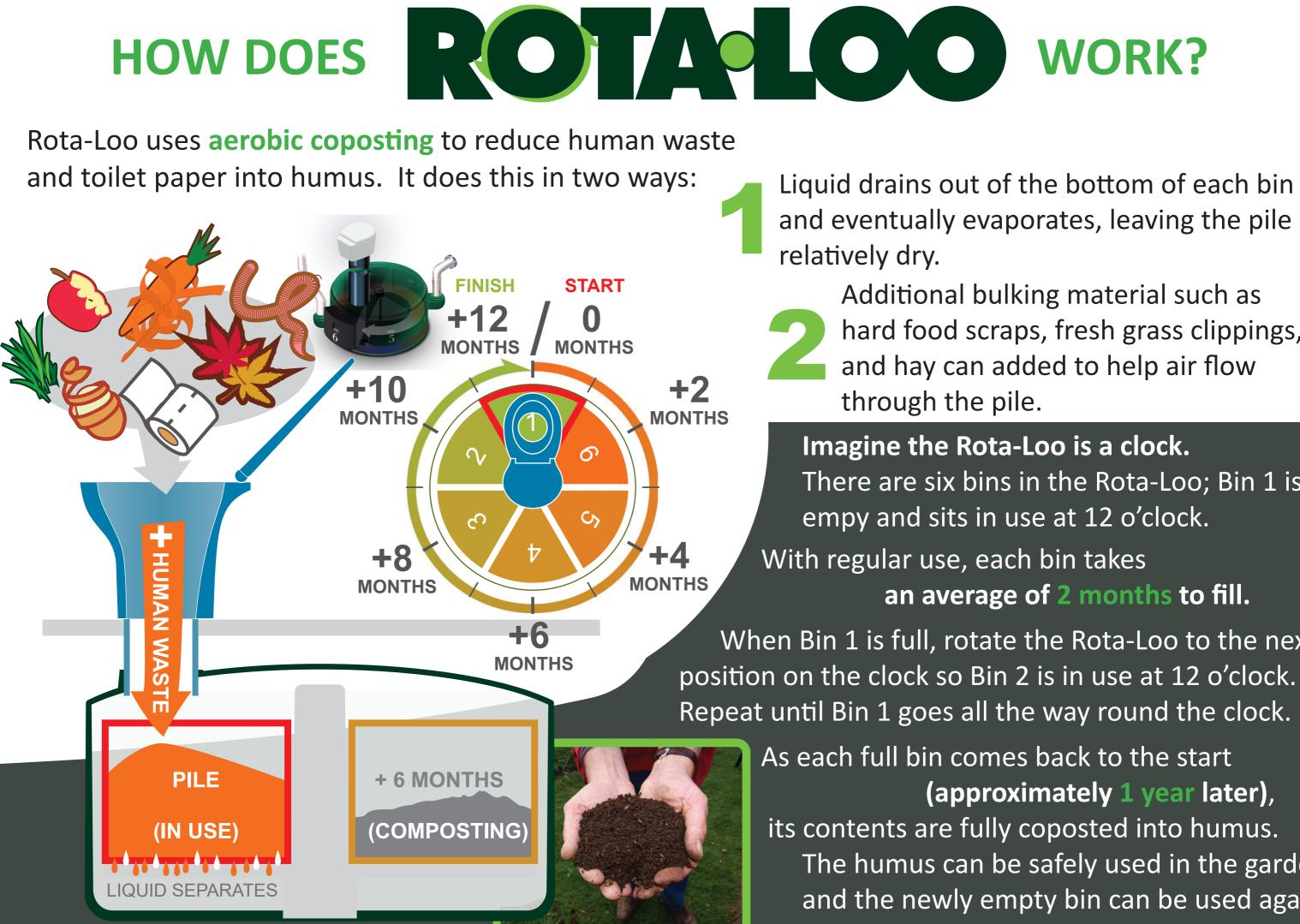
Liquid drains out of the bottom of each bin and eventually evaporates, leaving the pile
